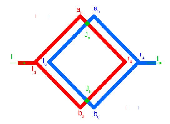
FIG. 7: The scheme of the DDCI with the loops shifted relative to each other. The boundaries of the Josephson junctions  $J_a$  and  $J_b$  do not coincide with the points  $a_u$ ,  $a_d$  and  $b_u$ ,  $b_d$ . Therefore the critical current may depend directly on the magnetic flux inside the loops.
