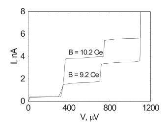
FIG. 4: Current-voltage characteristics of the DDCI structures with square side of the loops  $a \approx 4 \ \mu m$  measured at the temperature  $T \approx 0.44 \ K$  and different magnetic field  $B \approx 9.2 \ Oe$  and  $B \approx 10.2 \ Oe$ . Two extra steps correspond to the two additional Josephson junctions of the real DDCI at  $l_u$  and  $r_d$ .
