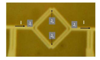
FIG. 2: The real structure used for the observation of the voltage jumps with the change of the quantum numbers of its two loops weakly connected by two Josephson junctions  $J_a$  and  $J_b$ . The two aluminium loops are shifted with respect to each other because of the simple technology of two-angle evaporation used in our work. The structure has two unnecessary Josephson junctions  $J_l$  and  $J_r$  because of this technology. Photo of 4  $\mu m$  aluminium loops is shown.
