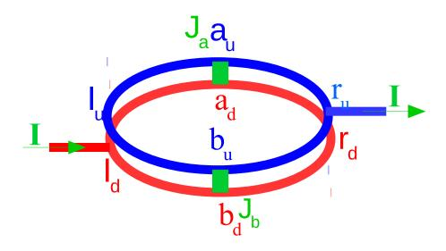
FIG. 6: The scheme of an ideal DDCI. The loops located one above the other and therefore the boundaries of the Josephson junctions  $J_a$  and  $J_b$  coincide with the points  $a_u$ ,  $a_d$  and  $b_u$ ,  $b_d$ . The critical current of such DDCI should not depend directly on the magnetic flux inside the loops.
