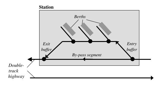
Fig. 2. Logical structure of a station
