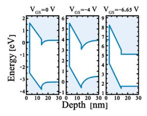
**Fig. 5** Band diagrams for 3 specific gate voltages (from zero to threshold voltage), calculated from the data of Fig. 4. The proposed method allows one to draw a band diagram for each single gate voltage (e.g., a diagram for each of the 150 spectra of Fig. 2) to visualize the evolution of the band diagram over the entire range of operation of the transistor.
