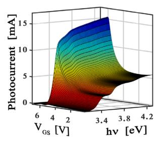
**Fig. 2** A series of 150 channel photocurrent spectra acquired from the high electron mobility transistor (HEMT) shown in Fig. 1 under a range of external electric fields. An external field was applied by applying voltage to the gate contact of the transistor ( $V_{GS}$ ), while the voltage between the drain and the source ( $V_{DS}$ ) was kept constant. In this figure,  $V_{DS}$  was  $0.1\,V$ .
