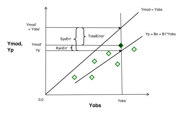
Figure 2. Graphical illustration of conceptual relationships among Yobs, Ymod, Yp, TotalError, and its components SysErr (systematic error) and RanErr (non-systematic error, or "noise"). Note that
