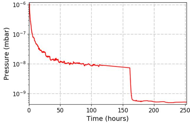
**Figure 7.** Chamber pressure of the entire system vs time, after equalisation at a bake-out temperature of  $130 \pm 1^\circ\text{C}$ . The temperature for the bake out was kept below that of the melting point of indium ( $\sim 157^\circ\text{C}$ ). After 160 hours the bake out ended and the temperature of the system returned to room temperature ( $\sim 21^\circ\text{C}$ ), and the pressure in the chamber reduced by roughly an order of magnitude.
