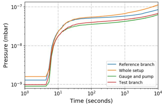
**Figure 8.** Rate of rise curves for the different sections of the vacuum system. The pressure before the rate of rise curve is not representative of the minimum achievable pressures but instead of the pressure in the chamber before the test was carried out.
