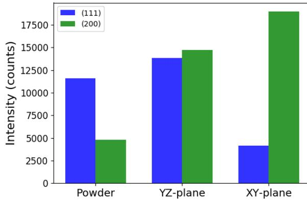
**Figure 3.** Comparison of the results from XRD tests on the unprocessed permalloy-80 powder and the sample produced with  $ED = 4.9 \text{ J/mm}^2$  along the XY and YZ-plane, respectively. The z axis is defined as the vertical axis of the sample. Each peak represents the intensity of the detected regions with the same crystallographic orientation. Although both phases are almost equally distributed on the YZ-plane, the (200) orientation dominates in the XY plane.
