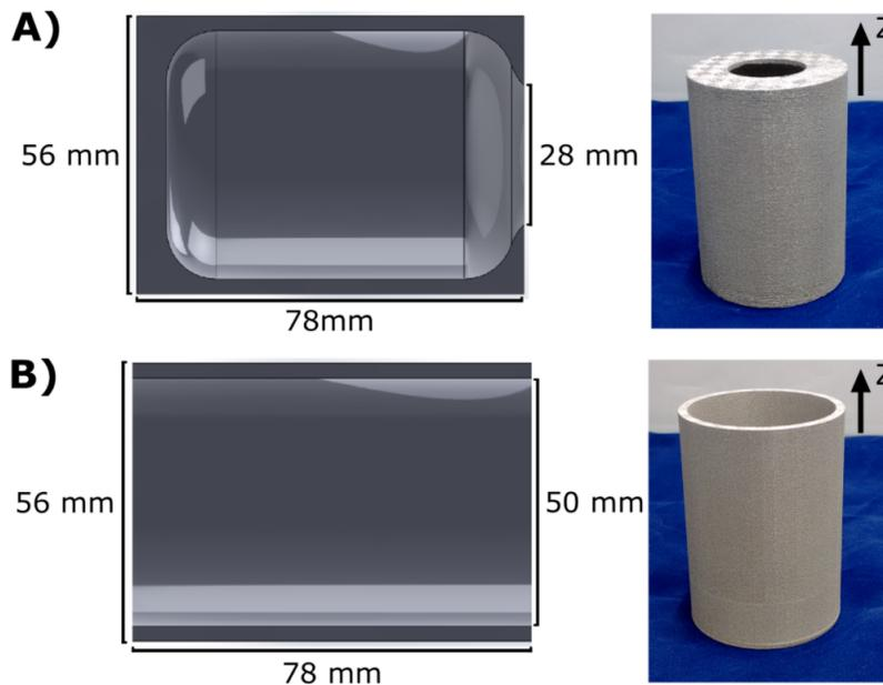
**Figure 1.** The 3D-printed magnetic shield structures used as test pieces. A) A cross section of the Z-Y plane showing the closed ended magnetic shield dimensions and a photo of the 3D-printed structure. B) A cross section of the Z-Y plane showing the open ended magnetic shield dimensions and a photo of the 3D-printed structure.
