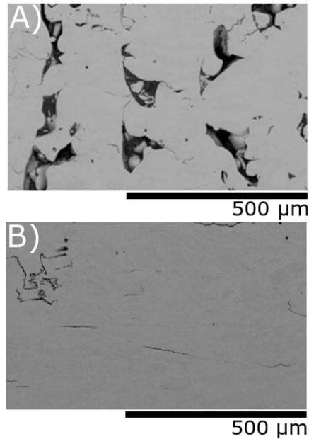
**Figure 2.** Pictures captured by a SEM on different 3D-printed samples revealing structural defects. A) Sample printed under non-optimal parameters with  $ED = 1.4 \text{ J/mm}^2$  and shows a large number of defects. B) Sample produced with under optimum parameters with  $ED = 4.9 \text{ J/mm}^2$  showing minimal defects.
