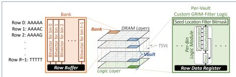
Figure 7: Left block: GRIM-Filter bitvector layout within a DRAM bank. Center block: 3D-stacked DRAM with tightly integrated logic layer stacked underneath with TSVs for a high intra-DRAM data transfer bandwidth. Right block: Custom GRIM-Filter logic placed in the logic layer, for each vault.
