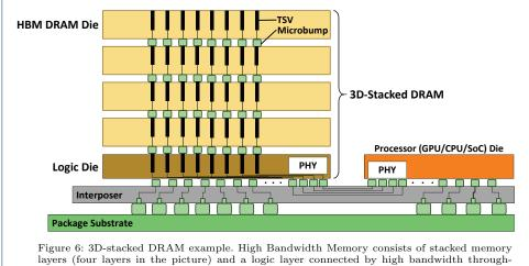
Figure 6: 3D-stacked DRAM example. High Bandwidth Memory consists of stacked memory layers (four layers in the picture) and a logic layer connected by high bandwidth throughsilicon vias (TSVs) and microbumps [2, 46, 59]. The 3D-stacked memory is then connected to a processor die with an interposer layer that provides high-bandwidth between the logic layer and the processing units on the package substrate.
