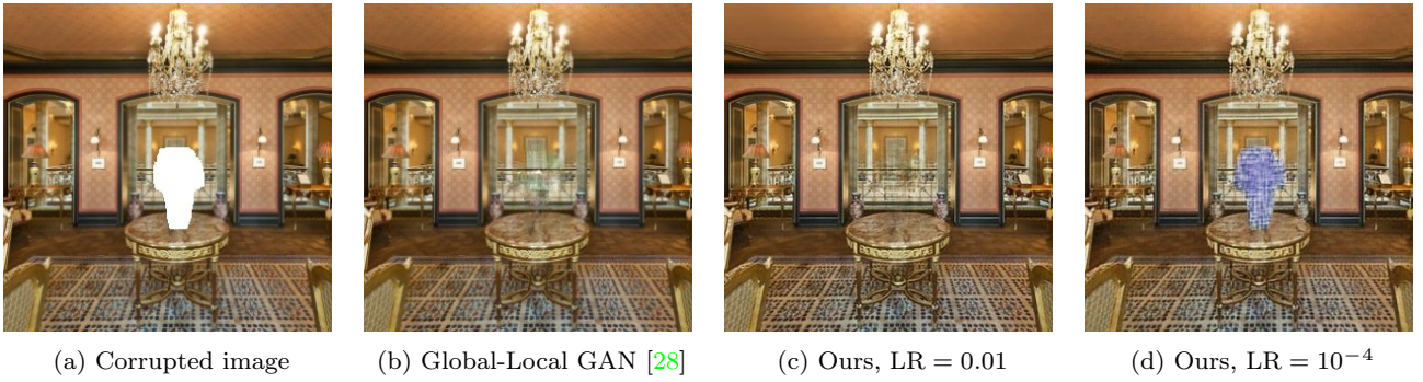
Fig. 10: Region inpainting. In many cases, deep image prior is sufficient to successfully inpaint large regions. Despite using no learning, the results may be comparable to [28] which does. The choice of hyper-parameters is important (for example (d) demonstrates sensitivity to the learning rate), but a good setting works well for most images we tried.
