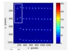
Figure 5: Framing camera mode (1  $\mu$ s x 100  $\mu$ s). 46/310 micropulses are shown. 3 MHz green component.
