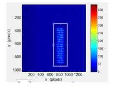
Figure 4: Vertical slow sweep image of 20 micropulses with 10-µs sweep range. Green at 3 MHz.
