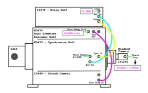
Figure 2: The Laser Lab streak camera wiring diagram. N:LGSHx and N:LGCTx are ACNET names for beam-synchronized VME-based timers.
