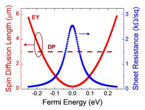
Fig. 3. Spin diffusion length modulation from EY (red) and DP (dark red) spin relaxation mechanism, and sheet resistance (blue) in single layer graphene. The calculations assume  $\Delta_{EY} = 12 \text{ meV}$  and  $\Delta_{DP} = 77 \mu \text{eV}$ .
