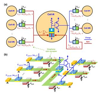
Fig.1 (a) Schematic diagram and (b) vision concept of GrSD CNN design. Synapse-to-neuron communication is in the spin current domain (red), which is controlled by the local electrostatic gating (black) while neuron-to-synapse communication uses charge voltage signals (blue). The weight programming circuits are electrically decoupled from the computation network.
