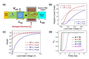
Fig. 7. (a) Neuron connected with a single graphene spin synapse (top view), the local gate dependence of the applied weights under (b) linear and (c) log scale. (d) Switching dynamics of FL PMA magnet under different applied weight value.
