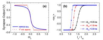
Fig. 6. (a) Output charge voltage as a function of input magnetization state simulated by HSPICE (blue) and its linear approximation (red). The linear function is used in the CNN simulations in the next section. (b) Averaged z-magnetization  $\langle m_z \rangle$  of magnet FL based upon 100 Monte Carlo simulations under different spin current pulse width.
