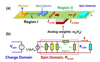
Fig. 4. (a) Schematic and (b) equivalent circuit model of graphene spin-diffusive synapse as a charge tunable voltage-controlled spin current source.
