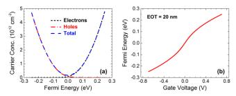
Fig. 2. (a) Carrier concentration dependence on relative Fermi energy in single layer graphene. (b) Fermi energy dependence on gate voltage,  $V_g$ , assuming an equivalent oxide thickness (EOT) of 20 nm, and a Dirac point at  $V_g = 0$ .
