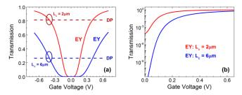
Fig. 5. (a) Gate dependence of spin transmission efficiency,  $T_s$ , on a linear scale for a single layer graphene spin-interconnect with EY or DP as the dominant spin relaxation mechanism (b) Log scale of  $T_s$  with EY spin relaxation only. The plots assume zero spin resistance at the detector magnet.
