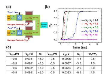
Fig. 8. (a) Schematic of cell with two input synapses, (b) Simulation of the corresponding switching dynamics (c) Weight programming table of the spin adder/subtractor.
