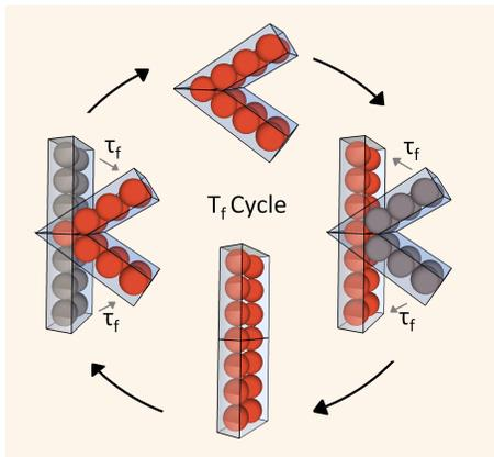
FIG. 1: (color online) Picture of the cycle showing the folding and unfolding of the motor's molecule. The total period of one cycle is  $T_f$  while  $\tau_f$  is the folding time. The motor is described with 14 centers of forces shown as atoms on the picture. The parallelograms are guides to the eye.
