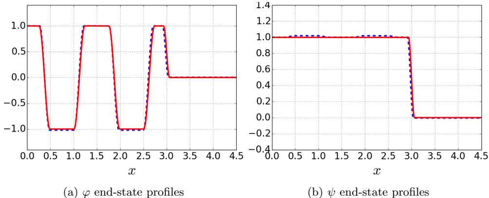
Figure 3: One-dimensional steady-state solutions obtained by solving the time-dependent model (14) with initial condition (41), the parameters (40), (42) with  $\mu = 10^{-3}$  (dashed blue lines) and  $\mu = 10^{-8}$  (solid red lines).
