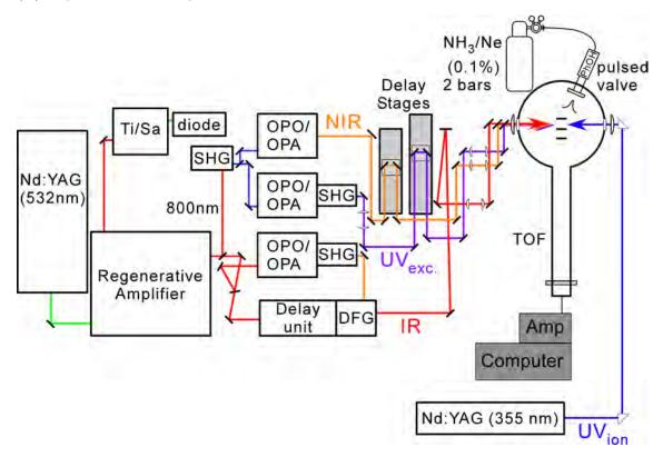
**Figure S1** A schematic diagram of the experimental setup of the picosecond time-resolved IR/NIR spectroscopy for PhOH– $(NH_3)_n$  clusters.
