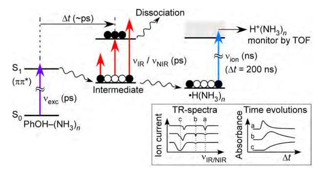
**Figure 2** Schematic diagram of the principle of picosecond IR/NIR spectroscopy of PhOH–(NH<sub>3</sub>)<sub>n</sub> clusters.
