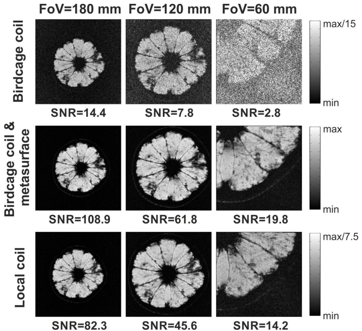
FIG. 4. Experimental demonstration of improved image quality with hybrid metasurfaces. MR images of grapefruit obtained with the birdcage coil only (top panel), with the birdcage coil and metasurface (middle panel) and with a 4-channel local receive coil (bottom panel) for different field-of-views (FoVs) corresponding to different voxels dimensions.
