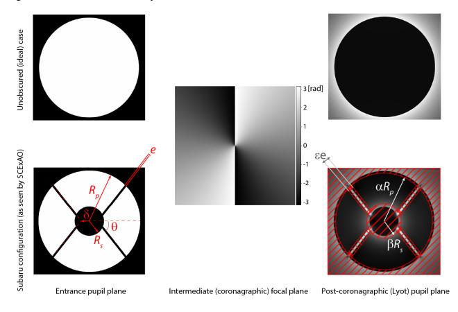
Figure 1. Principle of vector vortex coronagraphy for ideal (upper row) and Subaru-shaped (bottom row) telescope pupils, in the case of a topographic charge-2 phase mask. The Subaru pupil and SCExAO Lyot mask parameters shown here are detailed in Section §2.3 and Table 2.
