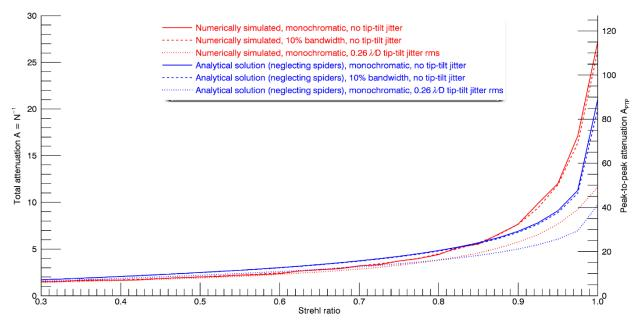
Figure A2. Numerically simulated (red) and analytical (Eq.12, blue) SCExAO vortex null depth performance predictions in function of Strehl ratio, in the diffraction-limited regime (SR > 0.3). Various leakage contributors (see Annex) are added to illustrate their respective impact on null depth. The right-hand side  $A_{PTP}$  vertical axis assumes a coronagraphic PSF geometric scaling factor  $A_{PTP}/A \sim 4.2$ , but this quickly loses validity for SR < 1.
