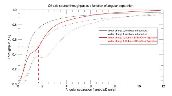
Figure A1. Vortex coronagraph throughput in function of angular separation for the ideal unobstructed pupil charge-2 and charge-4 cases (black curves), and the real Subaru-SCExAO configuration with a vortex chage-2 or charge-4 (red curves). The IWA (dashed red lines) of the current SCExAO charge-2 vortex is 1.7  $\lambda/D$  (70 mas).
