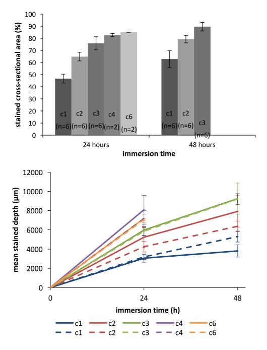
Figure 3: Study of contrast stain penetration. (top) percentage of stained cross-sectional area vs. immersion time. The error bars represent the standard deviation for each concentration. (bottom) mean stained depth vs. immersion time. The full lines represent the radial penetration, and the dotted lines the tangent penetration. n = 6 for each concentration.
