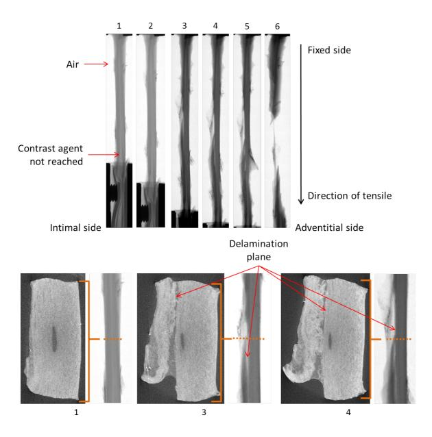
Figure 6: Rupture of a longitudinal sample with contrast agent (48 hours immersion, solution c3). (Top) successive radiographs illustrating the failure process, (bottom) cross-sectional views illustrating the microstructure at the initial state (1) and after rupture of the first elastic sheets (3-4). The location of the cross-section is indicated by dashed segments on the corresponding longitudinal views. Voxel size of 4 µm. Note that stain penetration was not complete for this sample.
