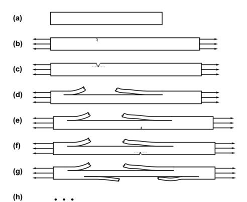
Figure 7: schematic representation of the damage initiation and propagation mechanism observed *in situ*. (a) intact sample, (b and c) initial radial crack, opening in mode I, (d) elastic recoil of the ruptured layers, causing a mode II longitudinal crack to form and propagate, (f, g, h...) the process repeats until complete failure of the sample.
