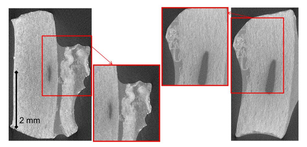
Figure 4: Visual comparison of the sharpness between 3D images obtained with samples immersed during 24 hours (right), and 48 hours (left) (4 µm voxel size).
