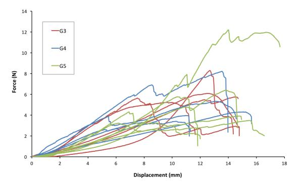
Figure 5: Mechanical effect of the contrast stain: force-displacement curves of all samples. G3 samples belong to the control group which was immersed in saline solution, G4 samples belong to the group which was immersed in 15g.L-1 SPT solution and G5 samples belong to the group which was immersed in 30g.L-1 SPT solution.
