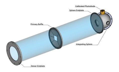
Figure 1. CAD drawing of baffle configuration
