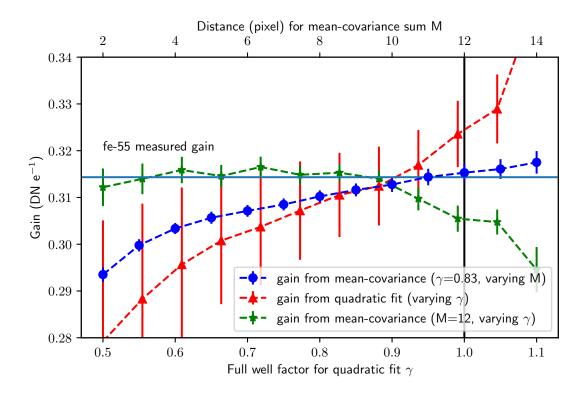
**Figure 7**. Measuring the camera gain using different methods from the same mean-variance data. In each case, errors are derived from the fitting covariance. The horizontal line shows gain as measured by Fe-55 for the same channel.
