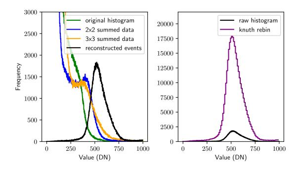
**Figure 4**. example Fe-55 histograms, constructed from 100 images, with  $V_{BB} = -60V$ . We compare raw images, summed in 2x2 and 3x3 regions, and simple event processed data (left panel). We demonstrate the use of optimal re-binning via Knuth's rule to improve histogram quality (right panel)
