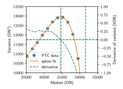
Figure 5. finding full well via a spline fit
