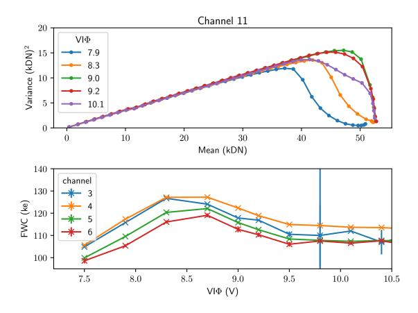
**Figure 9.** Measurement of full well as integration clock voltage  $V_{I\Phi}$  is altered. (above panel) the shape of mean-variance curves for various image clock voltages. (below panel) The measured full well capacity as image clock is adjusted. The vertical blue line shows the measured inversion threshold potential
