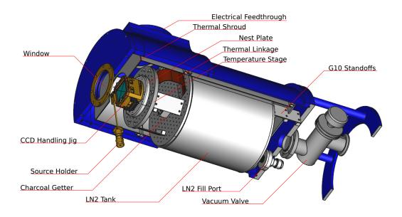
Figure 2. Partial cutaway view of the testing cryostat
