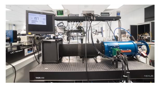
Figure 3. Photograph of optical test system in flat field configuration
