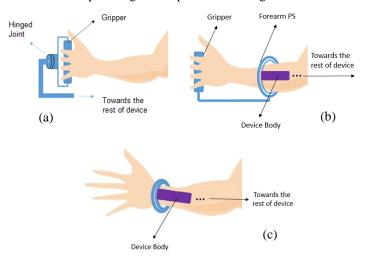
Figure 10. Example Concepts for Forearm PR: (a) MGA, (b) ARMin II, (c) Limpact
