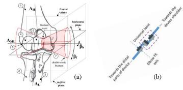
Figure 9. (a) Anatomy of Elbow and Rotation of the Elbow Axis [13], (b) A Design Concept to Allow this Motion
