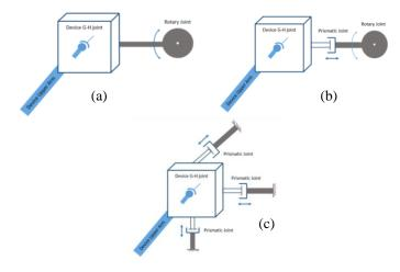
Figure 8. Design Concepts inner shoulder: (a) Single Revolute Joint (MGA), (b) Polar Structure (CLEVERarm), (c) Cartesian Structure.
