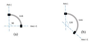
Figure 4 Angle between Consecutive Axes of Rotations as a Design Parameter
