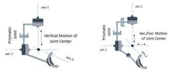
Figure 7. (a) Kinematics of ARMin II shoulder (b) Another Design Concept
