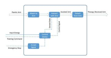
Figure 1. Functional Model of the Rehabilitation Device
