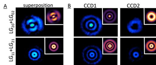
Figure 4. Mode superpositions  $\psi = \frac{1}{\sqrt{2}}(LG_{2,0} + LG_{0,2})$  and  $\psi = \frac{1}{\sqrt{2}}(LG_{1,1} + LG_{2,1})$  – **A**: The images show the intensity of the superposition, the inset shows the theoretical intensity distribution. **B**: Measured intensity distributions. The following two images show the output of the CCDs in the two output arms. As the modes have different mode numbers, they are sorted to different outputs of the interferometer.
