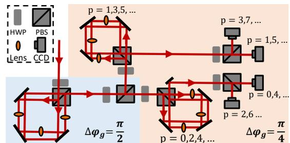
Figure 2. To sort higher mode-numbers, one could cascade the interferometers (a folded Sagnac-interferometer for long-term stability). Combining three such interferometers allows for sorting modes from  $p = 0$  to  $p = 3$ : The first interferometer (with blue background) sorts even and odd modes, while the subsequent two interferometers sort  $p = 0/p = 2$  and  $p = 1/p = 3$ , respectively. In our experiments, we show the results for both types of interferometers.
