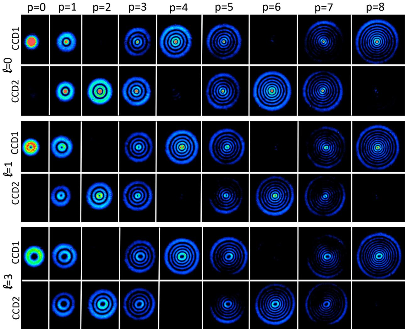
Figure 9. Experimental result for sorting  $p$  modes with constant  $\ell$  value by  $\Delta\varphi_g = \frac{\pi}{4}$ . From the two CCD outputs, we clearly see  $p=0,4,8$  and  $p=2,6$  be separated.
