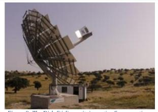
*Figure 8- The Dish-Stirling unit in routine Sun operations. We can see the very bright illuminated system focal plane.*
