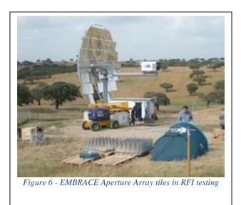
C. Commissioning and RFI testing : Demo Aperture Array tiles
