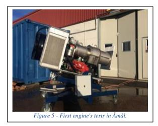
Before installing the Hybrid Stirling Engine, a solar version of a Stirling engine was installed in order to check the proper functioning of the system. The solar engine had been used before in Seville and was ready to run after checking and filling working gas and cooling water. No real commissioning of the engine was done since the main purpose was to check all other systems before moving on to the hybrid.
