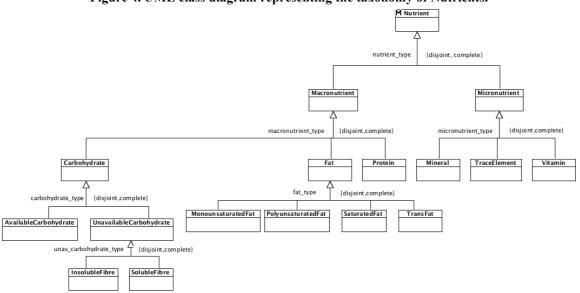
Figure 4. UML class diagram representing the taxonomy of Nutrients.
