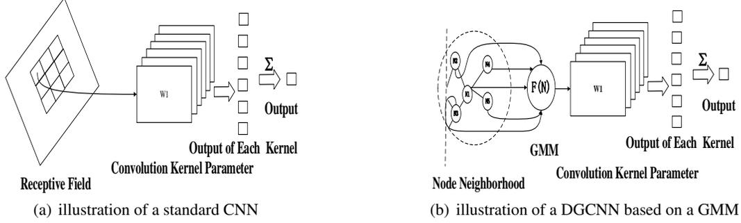
Figure 4: Convolutional Process Comparison between the Standard Image and a Node Neighborhood of the Graph Data
