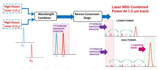
Fig. 1. Schematic illustrating simultaneous power combining and wavelength conversion.
