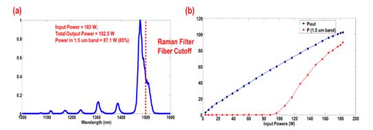
Fig. 3. (a) Spectrum at the output of the Raman filter fiber for a combined coupled input power of 183.4 W. (b) Power plot showing the evolution of the total output power and the power in the 1.5 micron band as a function of the combined input power.
