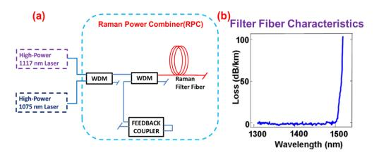
Fig. 2. (a) Architecture implementing the nonlinear Raman-based power combining. (b) Loss characteristics of the Raman filter fiber (from [11]).
