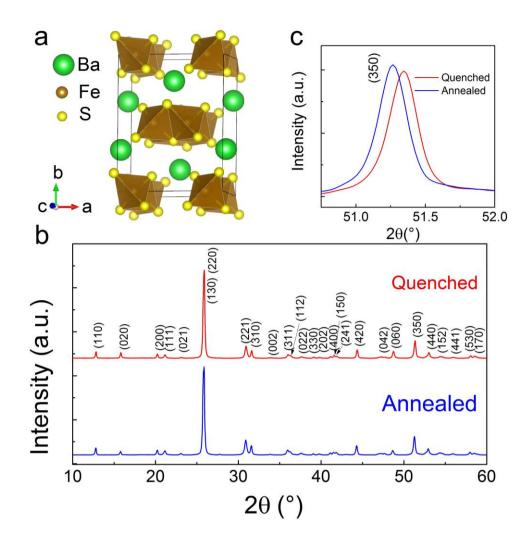
**Figure 1** (a) The schematic of the crystal structure of  $BaFe_2S_3$ . (b) Powder x-ray diffraction patterns for two samples with the quenching and annealing treatments. The powder samples were obtained by crushing the crystals. (c) An enlarged view of the PXRD patterns near (350) peak.
