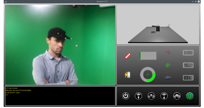
Figure 7: User interface of the framework. It is composed of 5 panels allowing to preview the shot, monitor the state of the drone and interact with it.
