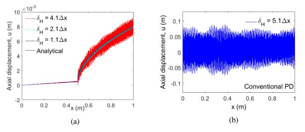
Figure 2: Spatial variation of displacement field: (a) local analytical solution and conventional PD solution with horizon sizes  $1.1\Delta x$ ,  $2.1\Delta x$  and  $4.1\Delta x$  (b) conventional PD solution with
