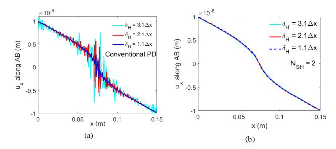
Figure 9: x-component of displacement along AB obtained through (a) conventional PD correspondence (b) sub-horizon based PD correspondence. Mesh and horizon sizes are
