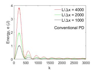
Figure 10: Frequency spectrum of conventional PD correspondence model
