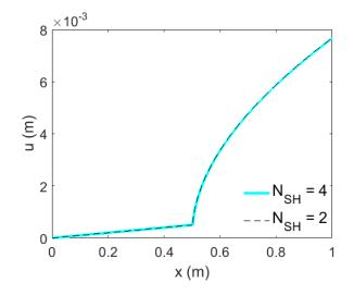
Figure 5: Spatial variation of displacement field obtained through sub-horizon based PD for horizon size  $\delta_{H} = 10.1\Delta x$  with different numbers of sub-horizons.
