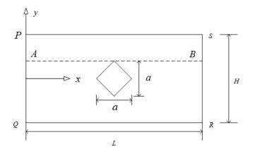
Figure 7: Geometry of the plate with hole and applied boundary conditions
