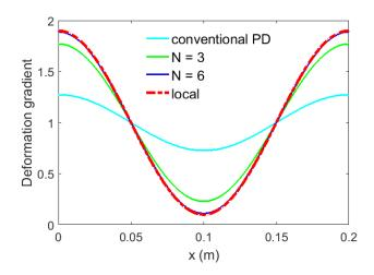
Figure 1: Local deformation gradient and its PD counterpart with and without correction. Correction orders considered are N = 3 and 6.
