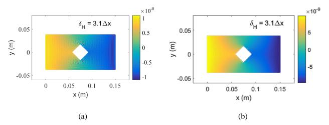
Figure 8: x-component of displacement obtained through (a) conventional PD correspondence (b) sub-horizon based PD correspondence. Mesh and horizon sizes are  $\Delta x = \Delta y = L/160$  and
