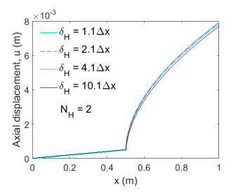
Figure 4: Spatial variation of displacement field through sub-horizon based PD for different horizon sizes; number of sub-horizons considered is 2.
