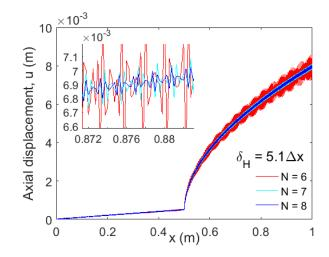
Figure 3: Spatial variation of displacement field obtained through corrected PD for horizon size  $5.1\Delta x$ . Displayed solutions correspond to correction orders N = 6,7,8.
