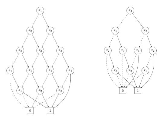
Figure 5: A 2-OBDD w.r.t. the variable ordering  $x_1, x_2, x_3, x_4$  and an FBDD for the function HWB<sub>4</sub>. Dashed lines represent edges with label 0 and solid ones edges with label 1. (See also [5].)
