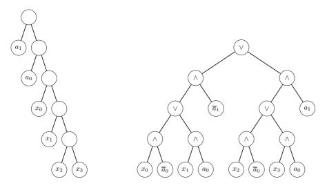
Figure 4: A right-linear vtree whose left-right traversal of the leaves corresponds to the variable ordering  $a_1, a_0, x_0, x_1, x_2, x_3$  and an SDD for the Boolean function MUX<sub>4</sub> w.r.t. this vtree.
