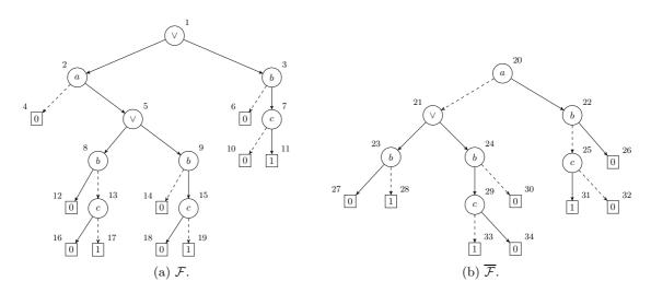
Figure 9: Unambiguous nondeterministic OBDDs  $\mathcal{F}$  and  $\overline{\mathcal{F}}$  representing the Boolean functions  $f(a, b, c) = (b \wedge c) \vee (a \wedge ((\overline{b} \wedge \overline{c}) \vee (b \wedge \overline{c})))$  and  $\overline{f}$ . Solid edges represent edges labeled by 1, dashed ones edges labeled by 0.
