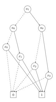
Figure 3: An OBDD for the Boolean function MUX<sub>4</sub> w.r.t. the variable ordering  $a_1, a_0, x_0, x_1, x_2, x_3$ . Dashed lines represent edges with label 0 and solid ones represent edges with label 1.
