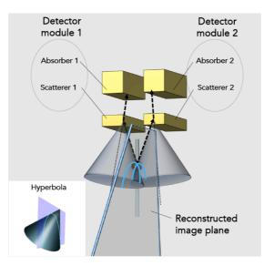
Fig.2: Reconstruction image plane. Intersection of the Compton cone with the reconstruction plane is defined by a hyperbola. Accumulation of hyperbolas generates the gamma image depicting the gamma-ray source.
