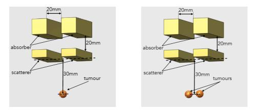
Fig.3: Schematics of the simulated setup for one (left) and two punctual tumours (right).
