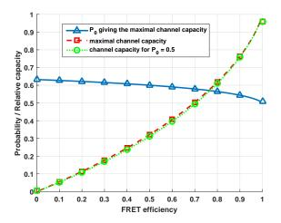
Fig. 9. The channel capacity as a function of FRET efficiency in two cases: for  $P_0 = 0.5$  (green dotted curve) and for the optimal  $P_0$  (red dashed curve). The value of the optimal  $P_0$  is additionally presented as a blue solid curve.
