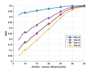
Fig. 7. Bit error rate for two communicating nanomachines as a function of their separation. Degree of labeling (DoL) of both nanomachines ranges from 2 to 9.
