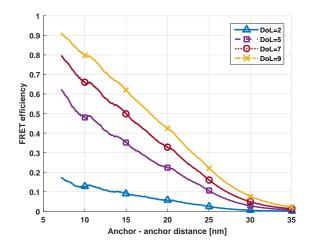
Fig. 4. FRET efficiency for two communicating nanomachines as a function of their separation. Degree of labeling (DoL) of both nanomachines ranges from 2 to 9.
