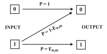
Fig. 1. FRET communication channel and transmission probabilities for bits '0' and '1'.
