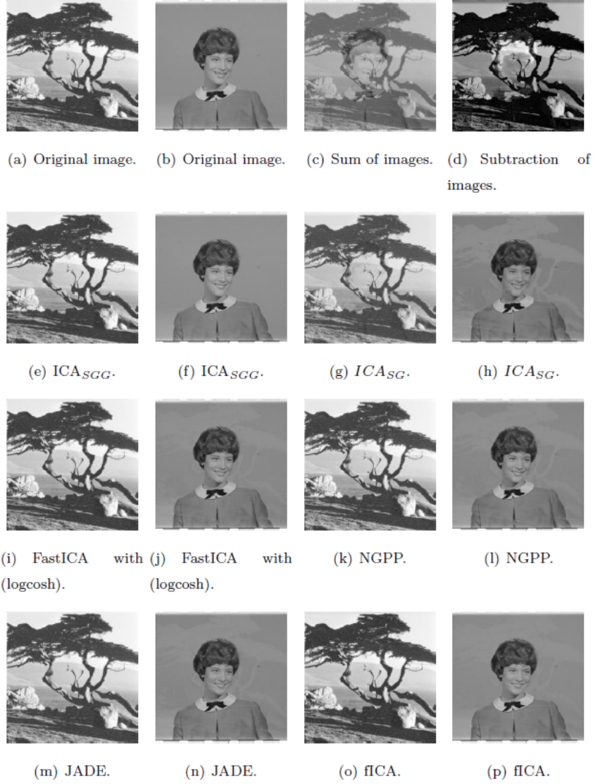
Figure 4: Results of image separation with the use of various ICA algorithms.
