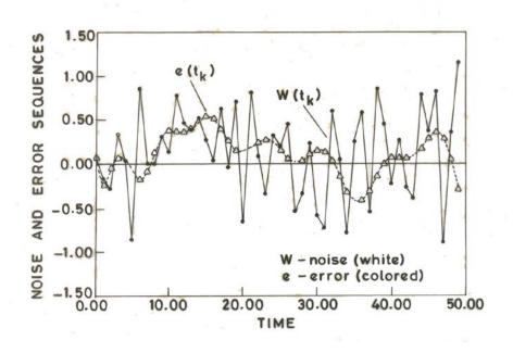
Figure 1 Orthogonal polynomial approximation: Peak SNR = 5 dB
