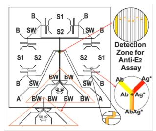
*Fig. 2. 6-channel mix, react, electrophoesis separation device for multiplexed immunoassays, ref 16.*
