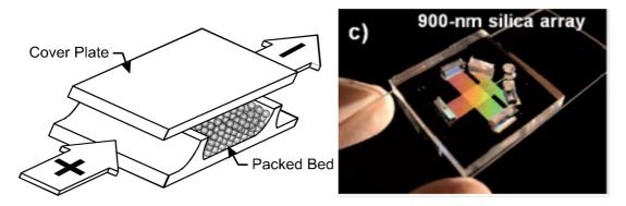
Fig. 3 left, Schematic of packed bed design for SPE, CEC, reaction beds; right, photo of crystalline particle bed for DNA separation, ref 39-44.
