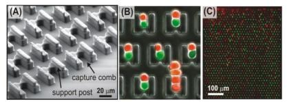
Figure 1. High-throughput cell pairing and fusion. (A) Device overview, (B) close-up of cell pairing, (C) Pairing over the entire array.
