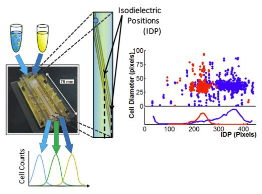
Figure 2. Iso-dielectric separation. A heterogeneous cell population (blue tube) is introduced in a microfluidic device where the cells encounter a spatial gradient in liquid conductivity and a dielectrophoretic force that pushes them across this gradient, until they reach their iso-dielectric point (IDP), where the force goes to zero and the cells cross over. At right are histograms of cell IDPs for unactivated (blue) and activated (red) human neutrophils.
