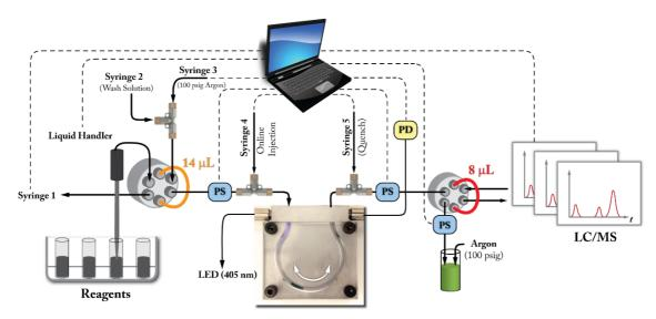
*Figure 2. Schematic of the automated droplet-based reaction screening platform. PS: phase sensor; PD: photodetector.*<sup>7</sup>
