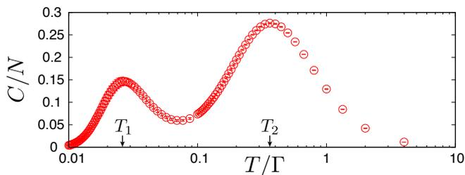
FIG. 11. (color online): Specific heat  $C/N$  of the AFM  $\Gamma$  model on the  $N = 24$  site cluster<sup>24</sup>, calculated by the typical pure quantum states approach<sup>30,31</sup>. There are two maxima in the temperature dependence of  $C/N$ . The error bars are the standard errors estimated by 32 random initial vectors.
