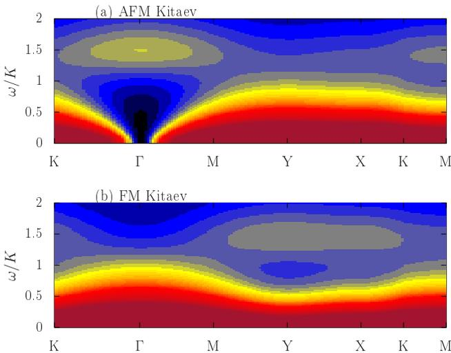
FIG. 18. Dynamic structure factor as obtained in Eq. (C6), for (a) the AFM Kitaev  $K > 0$ , and (b) the FM Kitaev  $K < 0$  models. Here we used  $\gamma = 0.25$ ,  $\Delta = 1.05K$  and  $g^2 T = 0.1K$ .
