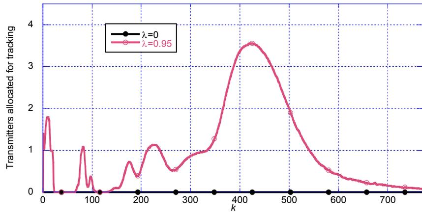
Figure 14 - Mean number of CPEs scheduled to transmit by the SR.
