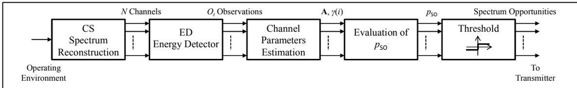
Figure 3 - Blocks in a cognitive radar.
