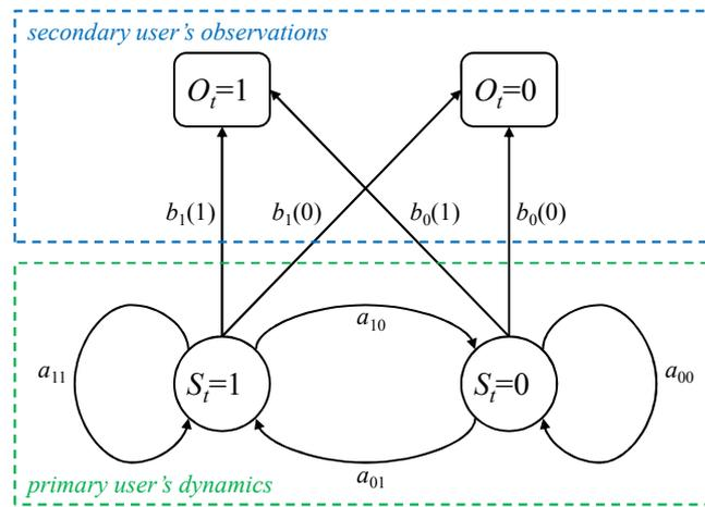
**Figure 4** - Hidden Markov Model representation for spectrum occupancy.
