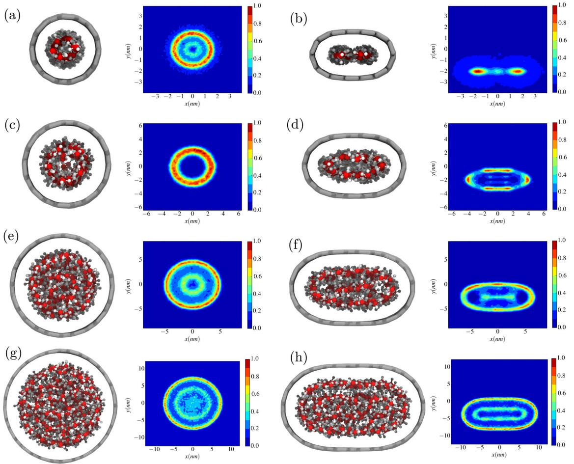
Figure 6: Left panels: snapshots of water molecules inside nanotubes along with radial ( $x$ - $y$ ) density maps of oxygens inside (a) (7,7), (c) (9,9), (e) (12,12) and (g) (16,16) carbon nanotubes with eccentricity  $e = 0.0$ . Right panels show the correspondent nanotubes with  $e = 0.8$ .
