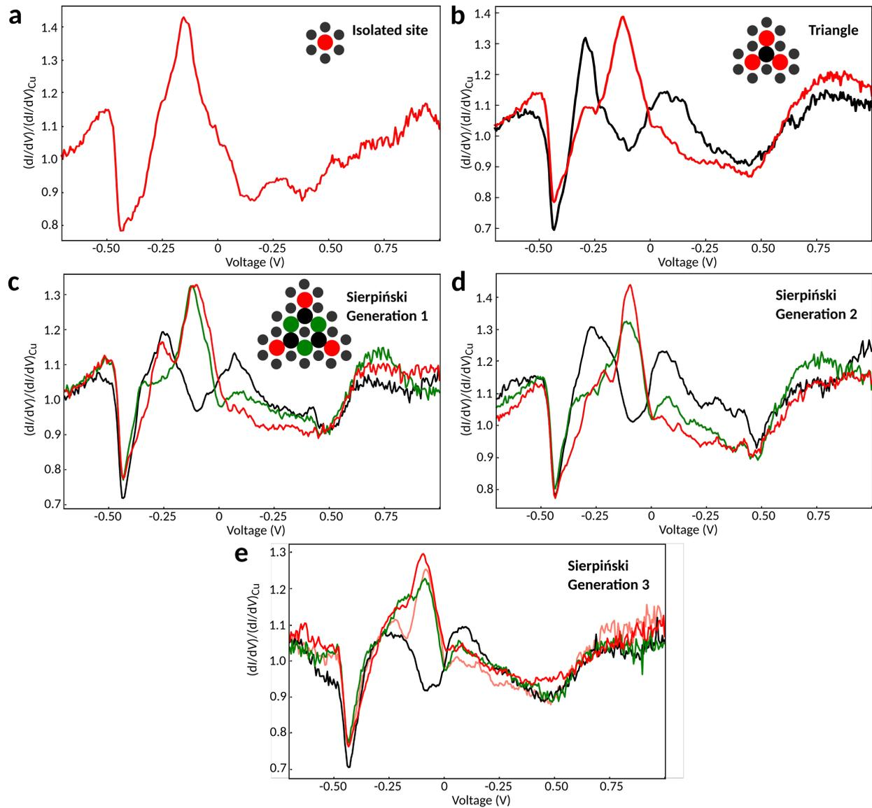
Figure S4. Normalized differential-conductance spectra over an isolated artificial atom site (a), a simple triangle (b, building block of the Sierpiński triangle), and a  $G(1)$  (c),  $G(2)$  (d) and  $G(3)$  Sierpiński triangle (e). The colors of the spectra correspond to the colors of the atomic sites indicated in Fig. S1a.
