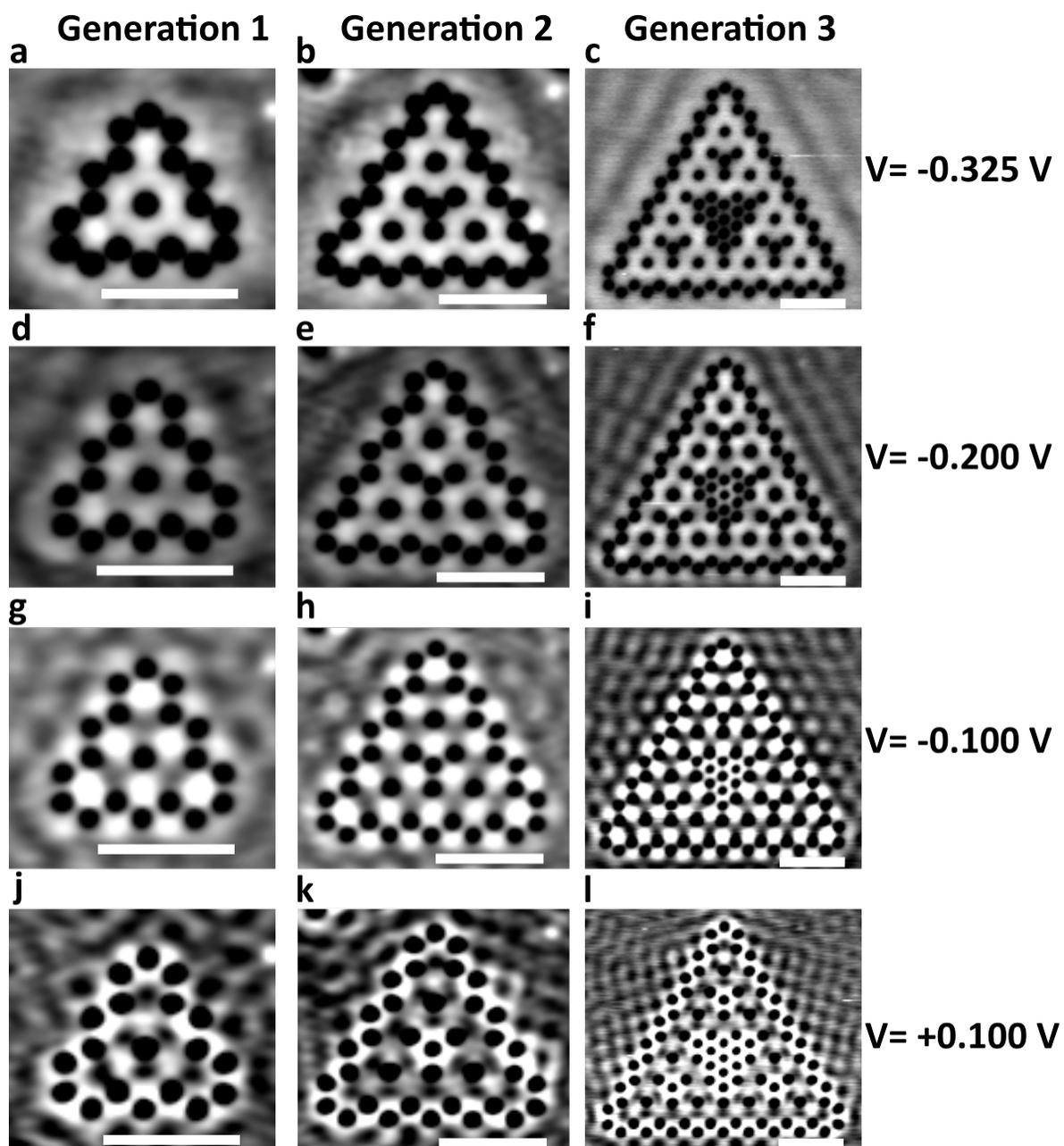
Figure S6. Experimental wavefunction maps for the first three generations acquired at  $V = -0.325$  V (a-c),  $V = -0.200$  V (d-f),  $V = -0.100$  V (g-i), and  $V = 0.100$  V (j-l). Scale bar: 5 nm.
