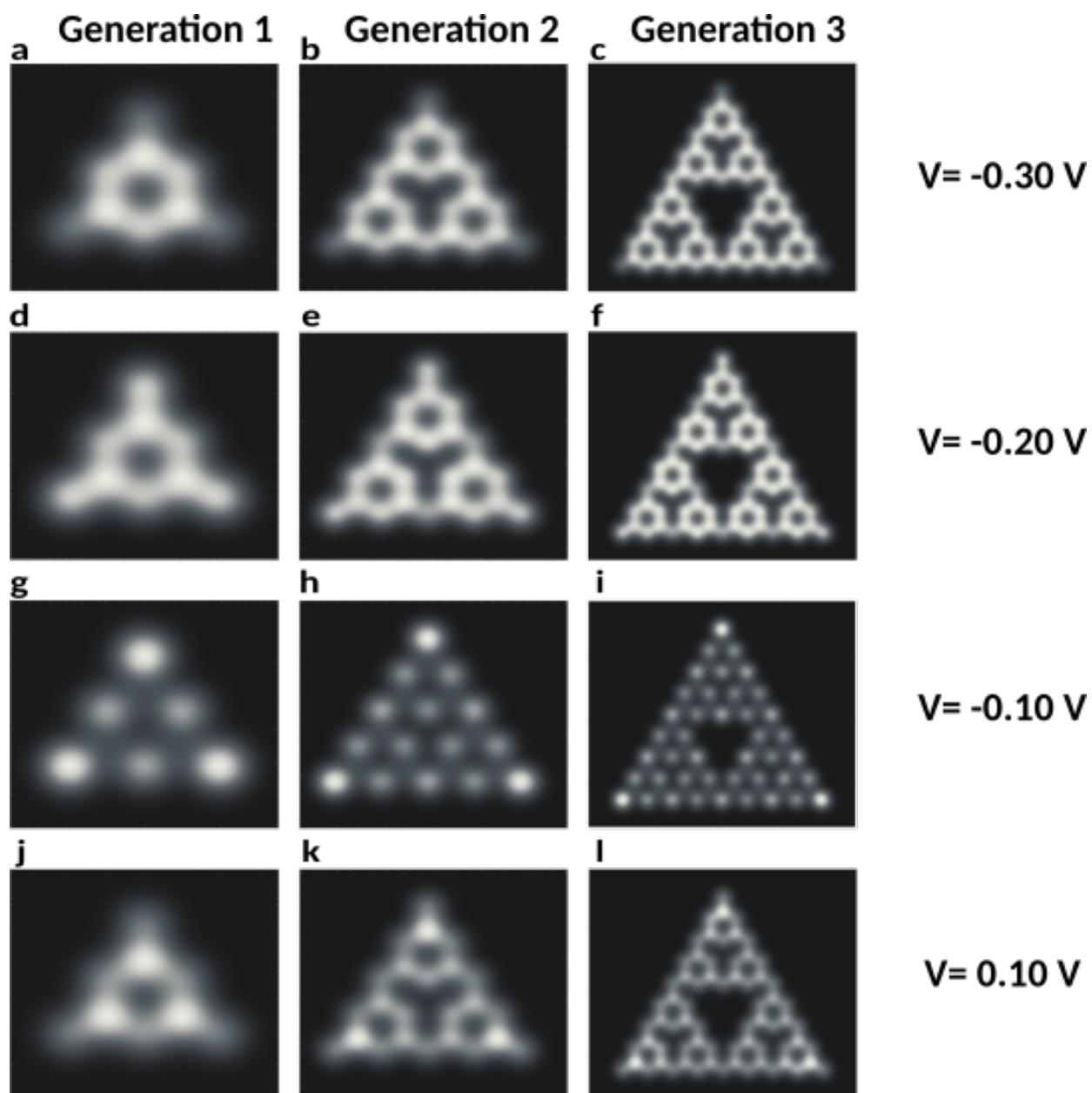
Figure S10. Wavefunction maps calculated within the tight-binding model for the first three generations of the Sierpiński triangle at  $V = -0.30$  V (**a-c**),  $V = -0.20$  V (**d-f**),  $V = -0.10$  V (**g-i**), and  $V = 0.10$  V (**j-l**).
