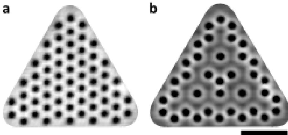
Figure S2. **a**, Scanning-tunneling-microscope image of a triangle with the size of a  $G(3)$  Sierpiński triangle, filled with a close-packed CO lattice. Imaging parameters:  $I = 1$  nA,  $V = 0.050$  V. **b**, Scanning-tunneling-microscope image of the resulting  $G(3)$  Sierpiński triangle after removing the redundant CO molecules by atomic manipulation. Imaging parameters:  $I = 1$  nA,  $V = 1$  V. Scale bar: 4 nm.
