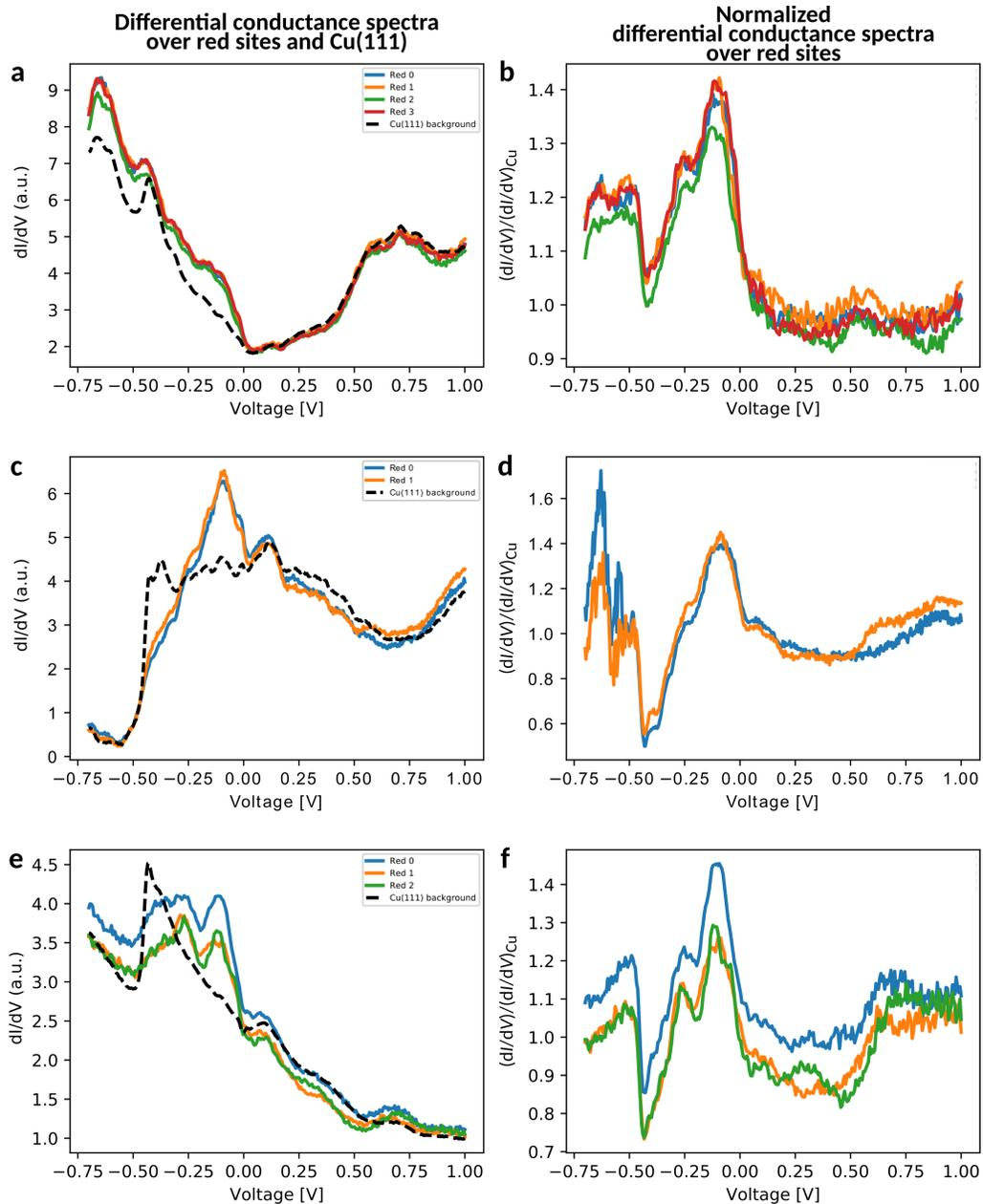
Figure S3. **a**, Differential-conductance spectra acquired over several equivalent red sites in a  $G(1)$  Sierpiński triangle (colored, solid lines) and an average of spectra over clean Cu(111) (black, dashed line). **b**, The spectra over red sites are divided by the average Cu(111) spectrum. **c-d**, **e-f**: same as **a-b** for tips characterized by a different spectrum on clean Cu(111). This normalization procedure leads to similar characteristic features, independently of the tip.
