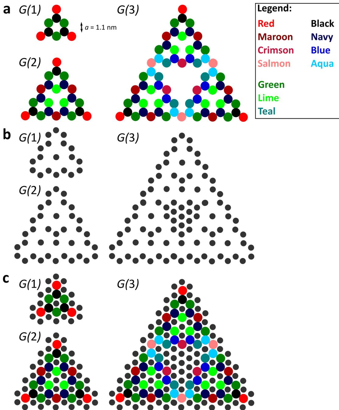
Figure S1. **a**, Tight-binding geometry of the Sierpiński triangle with honeycomb basis for the first three generations. **b**, Configuration of CO molecules, represented by grey disks, to confine the surface-state electrons of Cu(111) to the artificial atomic sites defined in **a**. **c** The tight-binding geometry of the Sierpiński triangle as well as the configuration of CO molecules.
