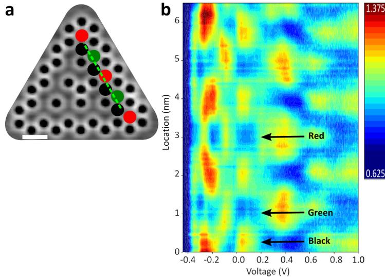
Figure S5. **a**, Scanning-tunneling-microscope scan of a  $G(2)$  Sierpiński triangle. **b**, Contour plot of 100 normalized differential-conductance spectra acquired along the green dashed line in **a**. The arrows indicate a black, green, and red site on the line.
