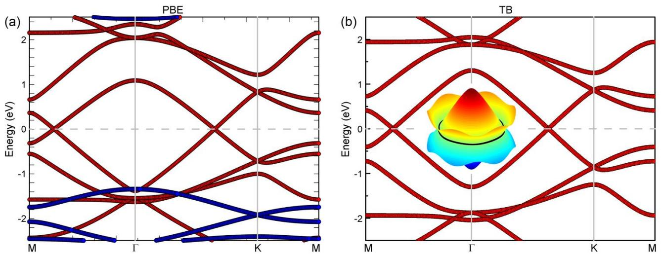
Figure 5. Orbital-projected band structure of  $H_{4,4,4}$ -graphyne monolayer from PBE calculations (a) and band structure of  $H_{4,4,4}$ -graphyne monolayer from TB calculations (b). In figure (a), the red (blue) dots represent the contributions from the  $p_z$  ( $s+p_x+p_y$ ) atomic orbitals of the carbon atoms. The red dots in figure (b) correspond to those in figure (a). The 3D band structure from TB calculations around the nodal line is presented as an insert in the figure (b).
