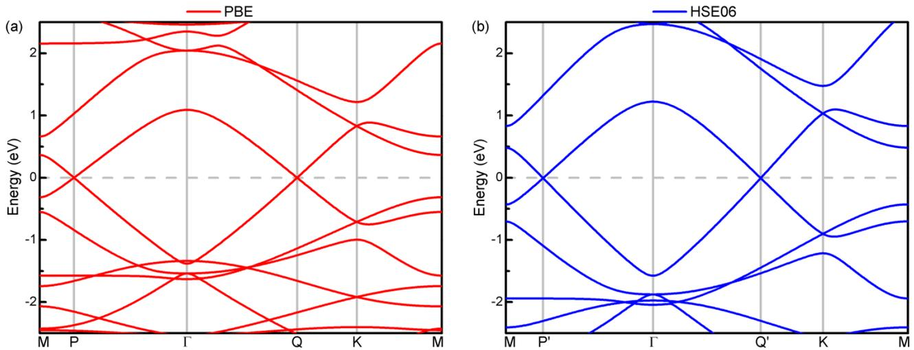
Figure 3. Band structures of the  $H_{4,4,4}$ -graphyne monolayer from PBE calculations (red lines, (a)) and HSE06 calculations (blue lines, (b)). The Dirac point in reciprocal space is labeled as P/Q/P'/Q'. The energy at the Fermi level was set to zero.
