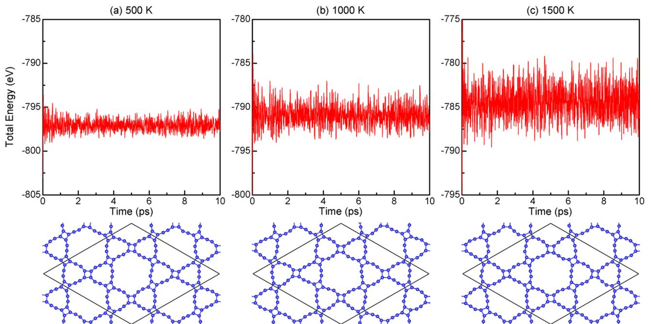
Figure 2. Fluctuations of total energy as function of simulation time and the corresponding snapshots of
