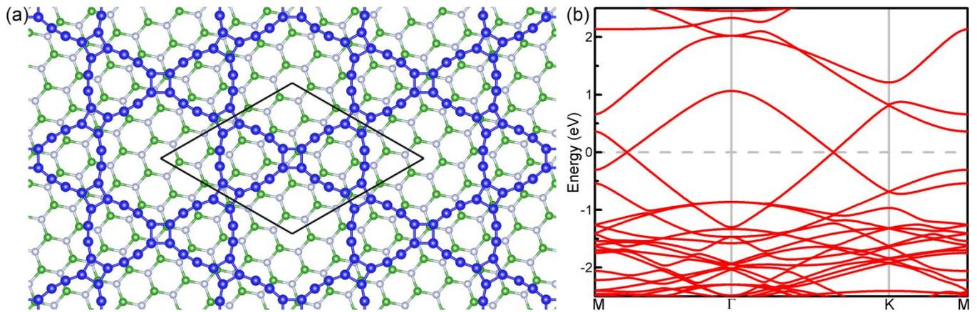
Figure 6. Schematic representation (top view) of  $H_{4,4,4}$ -graphyne/BN moiré superstructure (a) and corresponding band structure from PBE calculations (b). The blue/green/silver dots are carbon/boron/nitride atoms.
