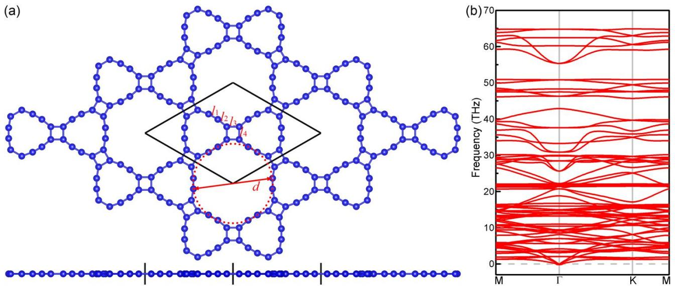
Figure 1. Schematic representations (top and side views) of  $H_{4,4,4}$ -graphyne (a) and its phonon spectrum along the high-symmetry points in the BZ (b). The blue dots are the carbon atoms. The four kinds of bond lengths are labeled  $l_1$ ,  $l_2$ ,  $l_3$ , and  $l_4$ , and the diameter of the circumcircle (red dotted line) of the 24 carbon ring is labeled  $d$ . The black box is the unit cell.
