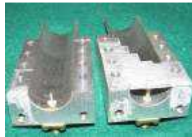
(B) Real horn with Septum polarizer disassembled.
