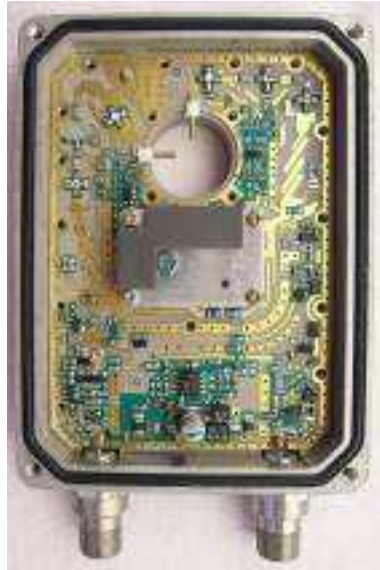
(A) LNBF with two ortho- gonal monopo- les.
