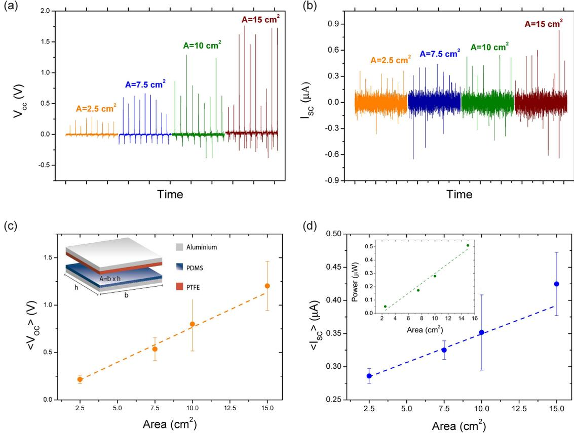
Figure 3: (a) Open-circuit voltage, (b) short-circuit current, (c) mean open-circuit voltage and (d) mean short-circuit current obtained for different areas of the triboelectric surfaces. The inset is the area dependence of the maximum power.
