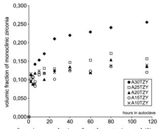
Fig. 4. Monoclinic phase fraction evolution for the yttria stabilized materials: influence of zirconia content.
