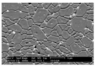
Fig. 2. A2.5Z-co, colloidal route. The very fine microstructure shows no aggregate at all.
