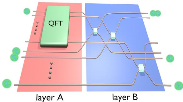
FIG. 1. Family of interferometers capable of witnessing genuine  $n$ -photon indistinguishability. QFT is the Quantum Fourier Transform acting on  $(n - 1)$  modes. Each output of the QFT is connected to a 50/50 beam splitter. As discussed in the main text, no mixture of extremal states with less than  $n$  indistinguishable photons can result in a probability of bunching  $p_b > \frac{2n-3}{2n-2}$ .
