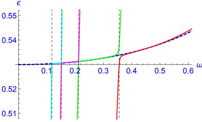
FIG. 10: A detail of Figure 7 showing various branches of the quasienergy (continuous colored curves), the corresponding resonance frequencies  $\omega_{res}^{(n)}$  (vertical dashed lines) and the asymptotic limit  $\epsilon_{asy} = \epsilon_0 + \epsilon_2 \omega^2 + \epsilon_4 \omega^4$  (blue dashed curve) for  $\omega \rightarrow 0$  according to (261), (264) and (265).
