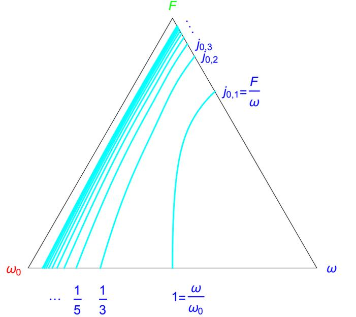
FIG. 6: The first ten resonance curves  $\mathcal{R}_n$ ,  $n = 1, \dots, 10$  in the triangular domain of variables  $\omega_0, \omega, F$ . They intersect the line  $F = 0$  at  $\frac{\omega}{\omega_0} = \frac{1}{2n-1}$  and the line  $\omega_0 = 0$  at  $\frac{F}{\omega} = j_{0,n}$  (the latter denoting the zeroes of the Bessel function  $J_0$ ), as will be shown below, see (183) and (232).
