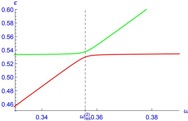
FIG. 8: The quasienergies  $\epsilon_i$ ,  $i = 1, 2$  for  $F = 1/2$  and  $\omega_0 = 1$  as functions of the frequency  $\omega$  in the neighbourhood of the resonance frequency  $\omega_{res}^{(2)} \approx 0.355776$ .  $\epsilon_1$  (green curve) has been calculated analytically and numerically as described in the text and  $\epsilon_2$  (red curve) has been chosen as  $\epsilon_2 = 3\omega - \epsilon_1$ .
