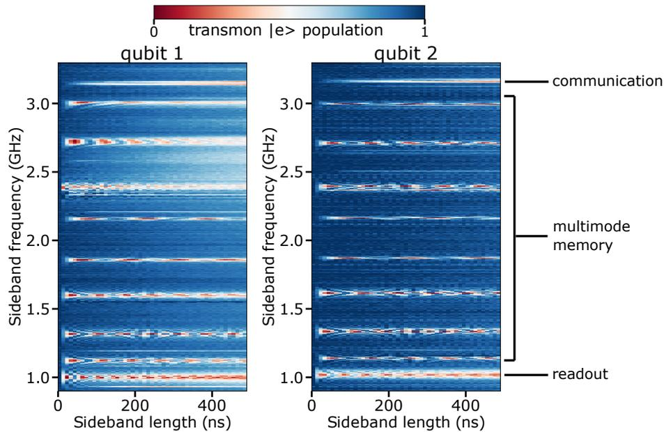
**Figure 7 | Full sideband Rabi spectrum of each qubit.** Stimulated vacuum Rabi oscillation with sideband frequency scan covering the band of all resonance frequencies of the resonators. The clean chevron patterns indicate that our transmons are free from spurious crosstalks. We can clearly identify ten chevron patterns corresponding to one readout resonator (lowest frequency), eight multimode memory resonators and one communication resonator (highest frequency).
