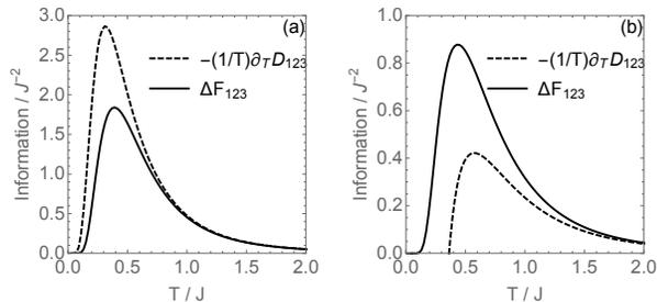
FIG. 3.  $\Delta\mathcal{F}_{123}$  and  $-(1/T)\partial_T\mathcal{D}_{123}$ , for Heisenberg system with three qubits at (a)  $B/J = 1, \alpha = 0.3$  and (b)  $B/J = 2, \alpha = 0.3$ . Note that the path denoted by subscript 132 and 213 have the same results.
