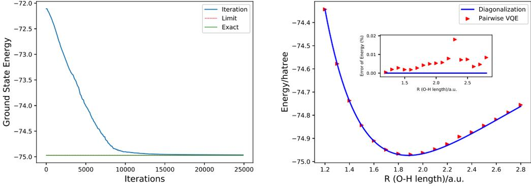
(a) Convergence of ground state energy of  $\text{H}_2\text{O}$  for fixed O-H bond length = 1.9 a.u., as number of iterations increases. The lines for exact ground state energy and for the limit almost overlap.
