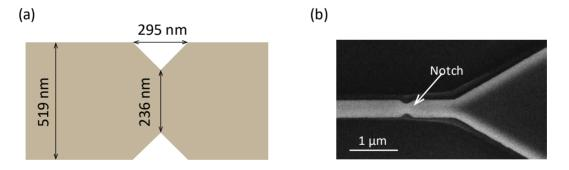
**Figure S7**. (a) Dimensions of the notch that is designed for coupling light from free-space into the nanobeam waveguide. (b) Scanning electron microscope image of the notch after fabrication.
