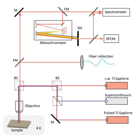
**Figure S3**. Complete schematics of the measurement setup. M, mirror; FM, flip mirror; SPCM, single-photon counting module.
