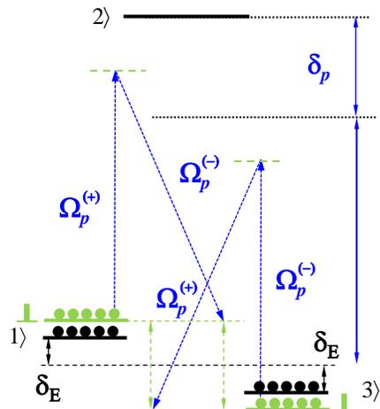
FIG. S4: **Laser coupling of pulsed magnetometry in the presence of a large background magnetic field (single beam configuration, WM field coupling can be similarly drawn)** The background field introduces a large nearly static Zeeman shift  $\delta_E$ . The very weak pulsed magnetic field introduces a minute medium magnetic dichroism change (i.e., field dependent two-photon detuning change) which can be detected by the WM method due to the large SNR enhancement.
