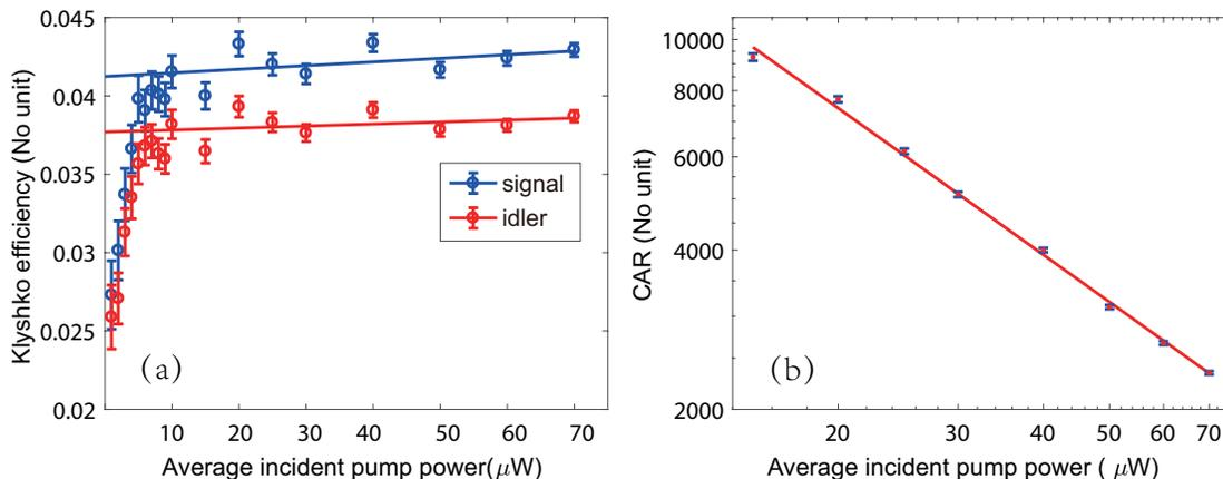
FIG. 2. (a) Klyshko efficiency for signal and idler and (b) CAR with respect to the average incident pump power. Symbols indicate the measured values, whereas the solid lines are fitted.
