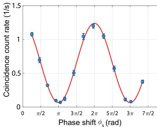
FIG. 5. Measured visibility (symbols) with respect to the phase change in the signal interferometer. The solid line represents a sinusoidal fit.
