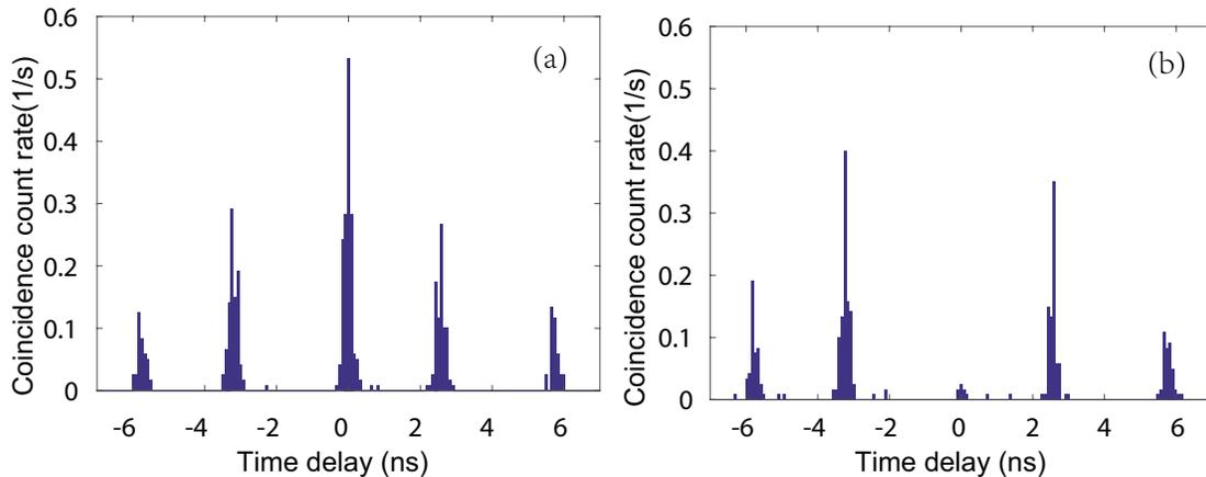
FIG. 4. Interferograms of coincidences between signal and idler shown in Figure 3(b) with respect to the time delay between their detection at two relative signal and idler interferometers' phases resulting in (a) maximal and (b) minimal amount of coincidences.
