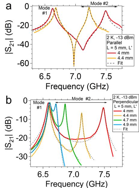
FIG. 4. Transmission spectra for the empty parallel (a) and the perpendicular (b) coupler configuration. The measures are performed at 2 K,  $P_{in} = -13$  dBm, zero magnetic field and for different lengths of the shorter slot ( $L' = 4, 4.4, 4.5, 4.7$  mm, see legends). Dashed lines correspond to the simulated spectra based on Eq. 6.
