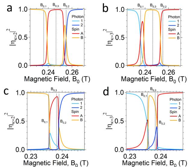
FIG. 7. Weight of the spin and photon modes in the hybridized system modes  $k = 2$  (a,c) and  $k = 3$  (b,d) calculated for the #A+#B case, both in the parallel (a,b) and in the perpendicular (c,d) configurations. Vertical dashed lines with labels show the positions of the resonant fields discussed in the text.
