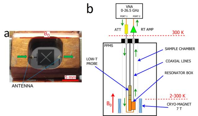
FIG. 3. (a) Photo of the shielding box with a perpendicular coupled DMR mounted inside. Green arrows show the path of the MW signal through the box, while the red arrow shows the direction of the static magnetic field  $B_0$ . (b) Sketch of the experimental set-up used in this work. Figure (b) is reproduced under Creative Commons Attribution License from Ref.<sup>3</sup>.
