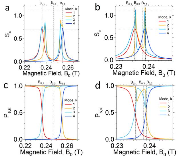
FIG. 8. Characterization of the hybridized modes in term of their modal entropy  $S_k$  (a,b) and the spin character  $P_{s,k}$  (c,d) as a function of the static magnetic field. The case of the  $\#A + \#B$  sample positioning discussed in the main paper (Fig. 2 and Fig. 3) are considered. Here (a,c) refer to the DMR with parallel coupling, while (b,d) refer to perpendicular one. Horizontal dotted lines in (a,b) correspond to  $\ln 2$  and to  $\ln 3$ , respectively.
